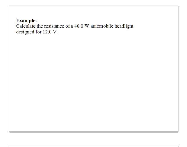
\*Note that this is the resistance when the bulb is burning brightly at 40.0 W. When the bulb is cold, the resistance is much lower. Since the current is high when the resistance is low, <u>lightbulbs</u> burn out most often when first turned on.
