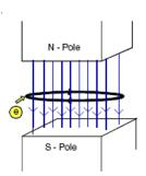
The permanent and induced magnetic fields interact to force the electron in a certain direction as shown.
