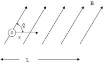
This charged particle, q, will constitute a current if 'n' particles pass a certain point in a given time  $\Delta t$ .
