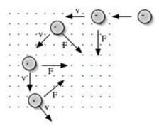
Note the force on the electron (using left hand rule). Since the force is always perpendicular to the velocity, the magnitude of the velocity does not change but the particle changes direction and moves in a circular path, with a centripetal acceleration. The force is directed toward the centre of the circle at all points. So in this case the electron will move in a counterclockwise circular path.
