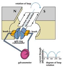
The <u>commutator</u> allows current to flow continuously in one direction. This kind of current is called DC or direct current. The kind of direct current from a generator is not exactly the same as that from a chemical source like a battery (because the current still drops to 0).
