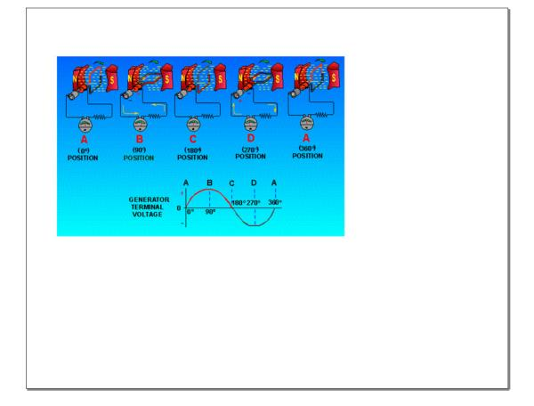
Notice that in position B current is <u>maximum</u> in one direction. The current is induced as shown because of Lenz's law.
