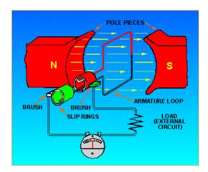
Slip rings rotate with the loop while the brushes remain stationary. At the position shown here the conductor is not cutting across any field lines so no current is induced. As the conductor rotates through 360° current is induced while field lines are being cut as shown below.
