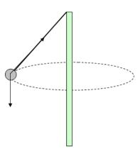
The acceleration points horizontally toward the centre of the ball's circular path. The vertical component of the string tension balances the ball's weight mg. The horizontal component of the string tension,  $F_{TX}$ , is the force that produces the centripetal acceleration toward the centre.
