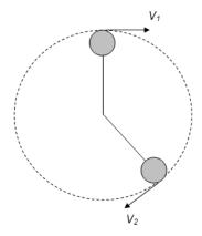
An object revolving in a circle is continuously accelerating even though the speed v, remains constant.
